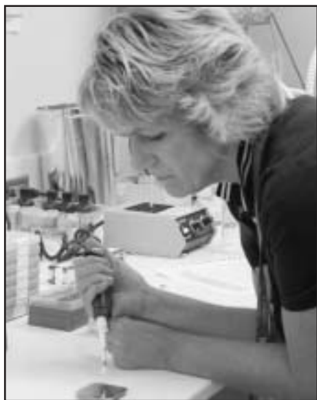
Teresa Hayes, from Wauneta-Palisade Public Schools, visited the Protein Structure Core Facility. Here, she learns to spot peptides onto a plate before determining its molecular weight by MALDI-tof (Matrix Assisted Laser Desorbed Ionization by time of flight).
